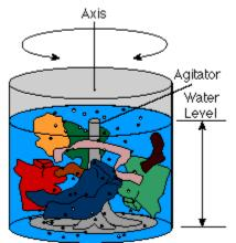
Figure 3-10 Clothes Washer Vertical Axis Configuration
