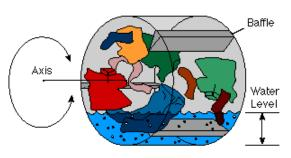
Figure 3-11 Clothes Washer Horizontal Axis Configuration
