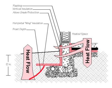
Figure 3-1 Heat Exchange Occurring at an insulated building foundation
