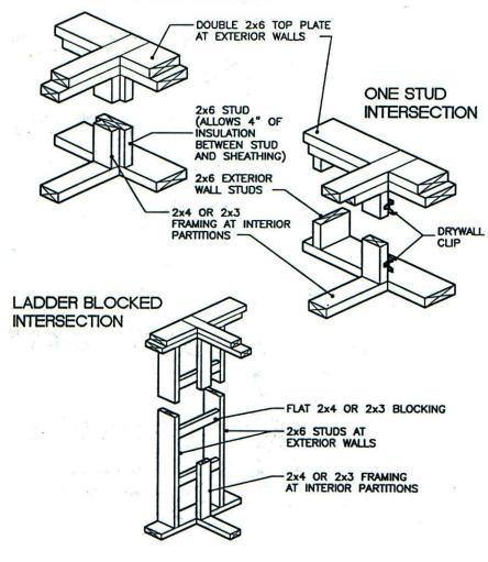
**Figure 3-6 Construction Details for Easy of Insulation** (Source: Washington State Energy Code Builder's Field Guide)
