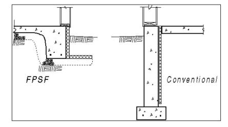
Figure 3-2 A frost protected shallow foundation in comparison to a conventional house foundation.
