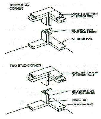
Figure 3-5 Corner Construction (Source: Washington State Energy Code Builder's Field Guide)
