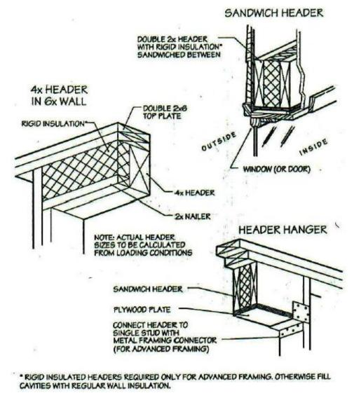
Figure 3-4 Insulated Headers (Source: Washington State Energy Code Builder's Field Guide)
