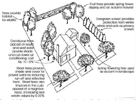
Figure 2-2 Tree Placement to Reduce Heating/Cooling Loads Naturally
