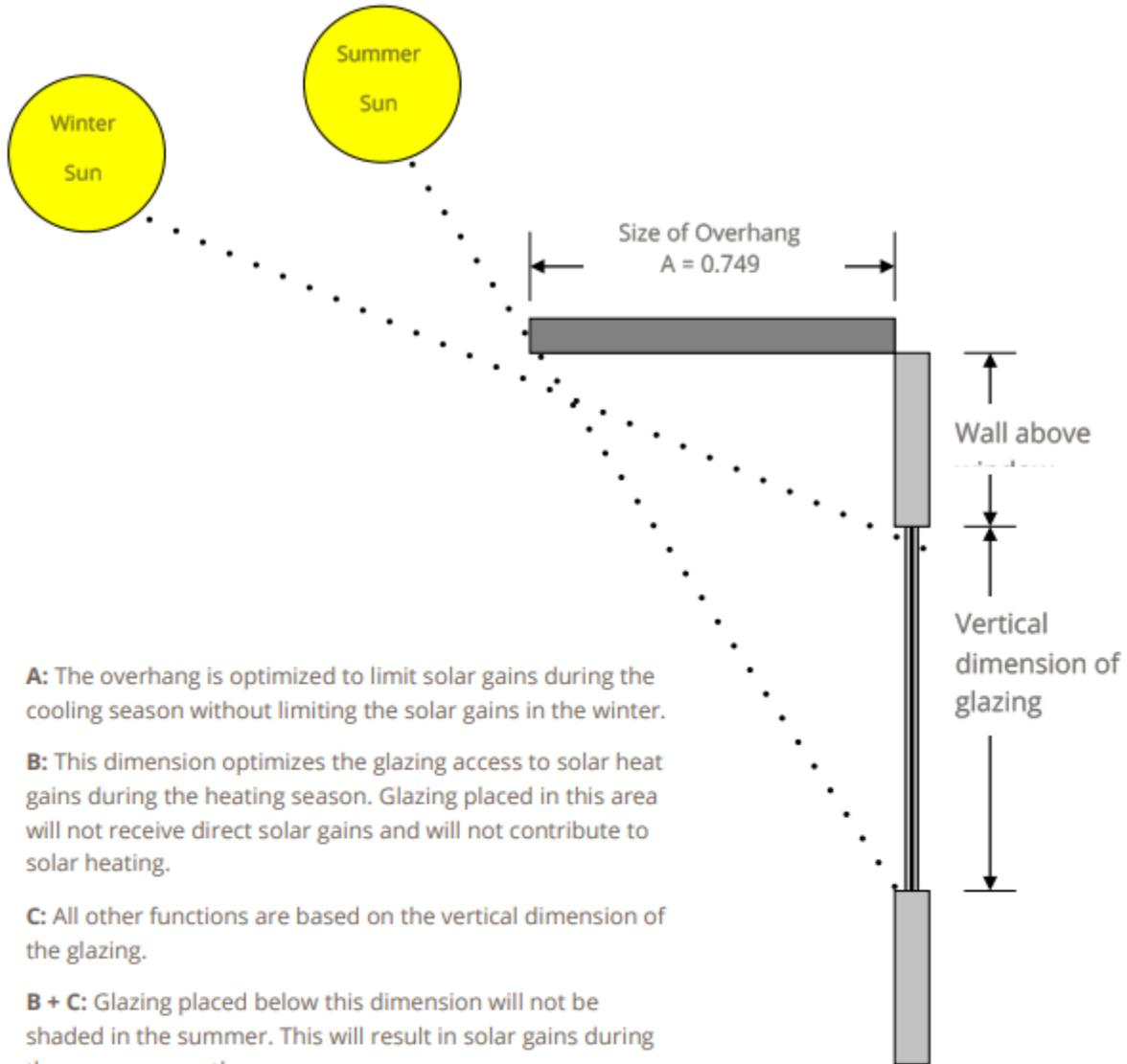
This figure is for buildings built in Seattle, or other sites at 47.5 degrees latitude. The effectiveness of the shading diminishes if the building orientation changes. Within 30 degrees of due south, this formula will provide relatively good results. East and West facing glazing require shading by other means such as exterior blinds, or landscaping.
