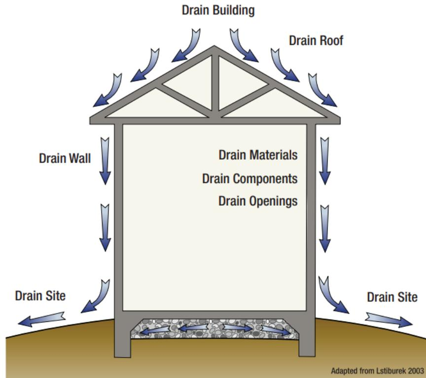
**Performance Requirement:** Comply to builder requirements described in the EnergyStar Water Management System checklist section 2 water-managed wall assembly, see resources below.
