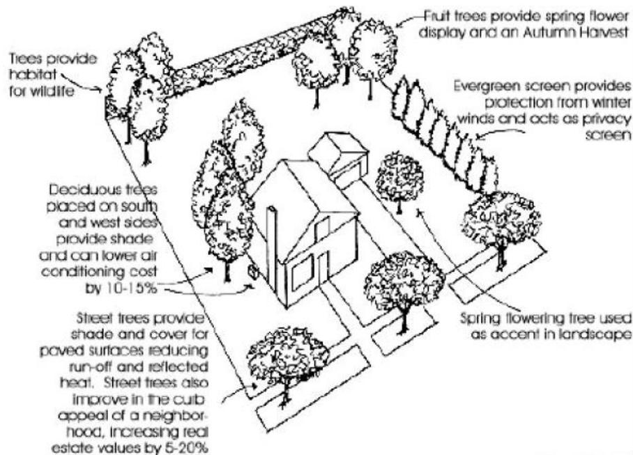
Figure 2-2 Tree Placement to Reduce Heating/Cooling Loads Naturally
